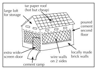
The PROJIMO workshop first opened on the back porch of an old house. A year later a new shop was designed and built with community participation, and some outside funding. It is 8 x 12 meters. Two walls are screened, on the sides the rain is least likely to blow in. A large loft provides storage space and helps to keep the work area below cooler. The new shop is already too small!
